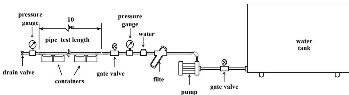
Fig. 1. Laboratory experiment layout.
